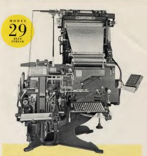
CONTINUOUS mixed composition is provided for the efficient production of intricate matter for some kinds of book, commercial and advertising work. With the flick of a conveniently-placed lever, the operator can assemble matrices from two adjacent magzines without shifting magzzines, of which a maximum of four are available.
